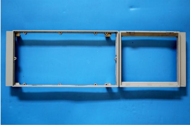
Replace the original bezel with the modified bezel. Install the subpanel and keyboard PCB A1A1 to the new bezel. Replace the front dress panel, retaining nuts, “Level” knob, and “Intensity” knob.
