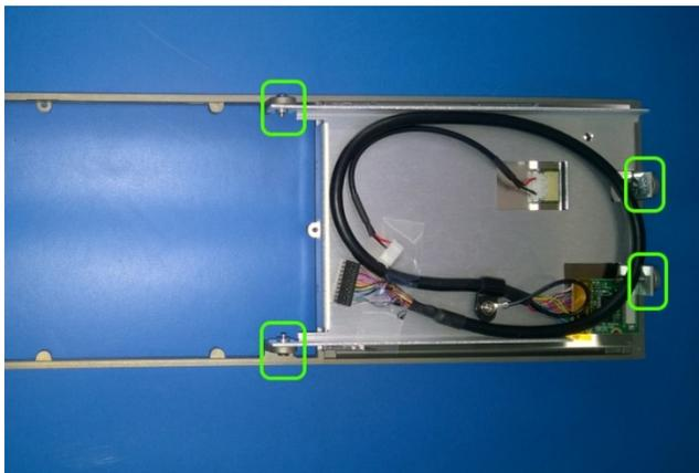
In the kit that you received, the LCD panel assembly is installed in the bezel for shipping purpose. It needs to be removed for installation. (6.5” VGA panel assembly shown)
