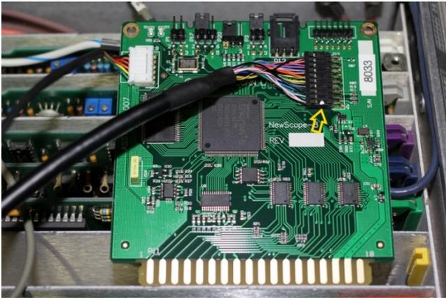
Feed the display link cable and display board control cable through the venting holes into the A3 card cage.
