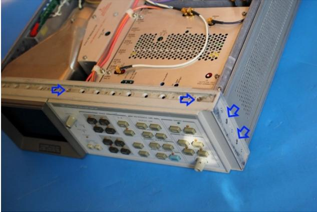
Remove the plastic trim strip on the top of the unit by inserting a small flat screwdriver into the slot and lifting upwards. Remove two screws located under trim strip.
