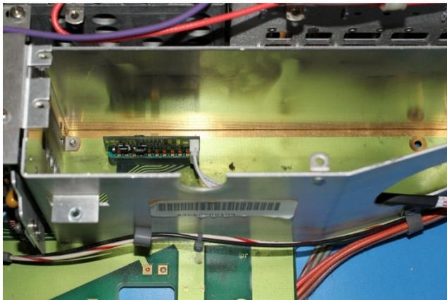
Plug the 6-pin end of the Power Plug Board control cable on the Power Plug board. Install the Power Plug board in A1XA3P1. Note that pin 1 is facing the front of the unit.
