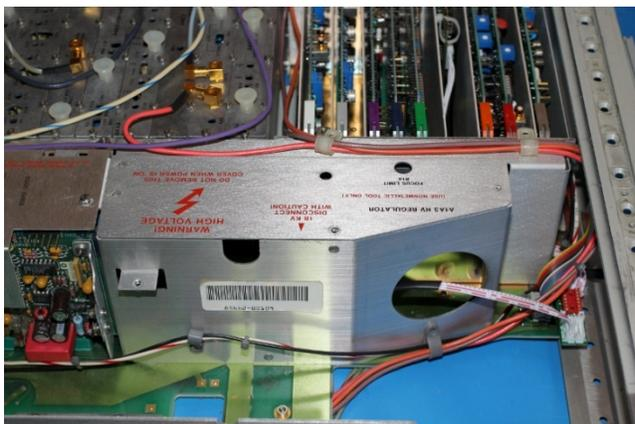
Reinstall the A1A3 shielding cage cover. Ensure the display link cable and the display board control cable pass in front of the A1A3 cage.
