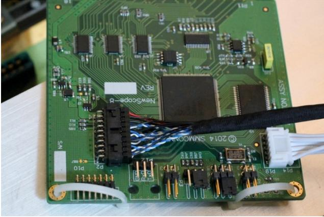
Make two loops with wire ties. These will be the extraction aid should you need to remove the board later. Rest the loop in the PCB notch.
