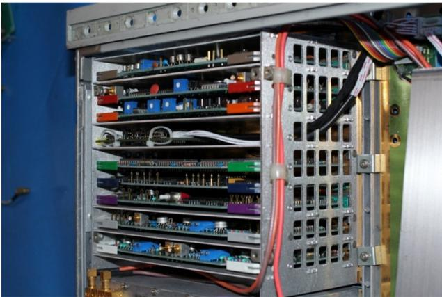
Install the main board into the A3A4 card cage slot, route the display link cable and the display board control cable between the A3 card cage and the A1A3 shielding cage to the LCD panel area.
